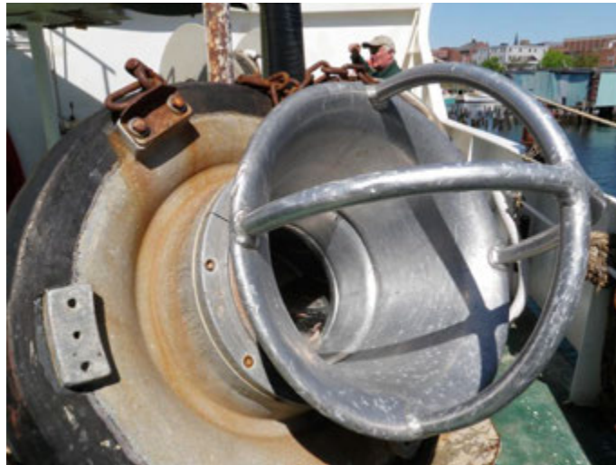
Figure 1. A bell, the beginning of the pumping process on a herring vessel
