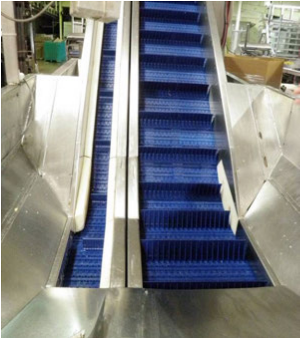
Figure 28. The dual conveyor belt picks up fish in small and large increments, to be used to fill the hoppers to the desired weight for packagaing.
