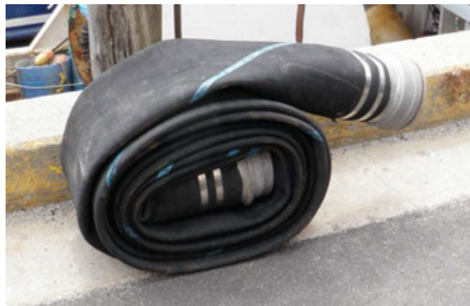
Figure 2. Example of tubing used for pumping fish
