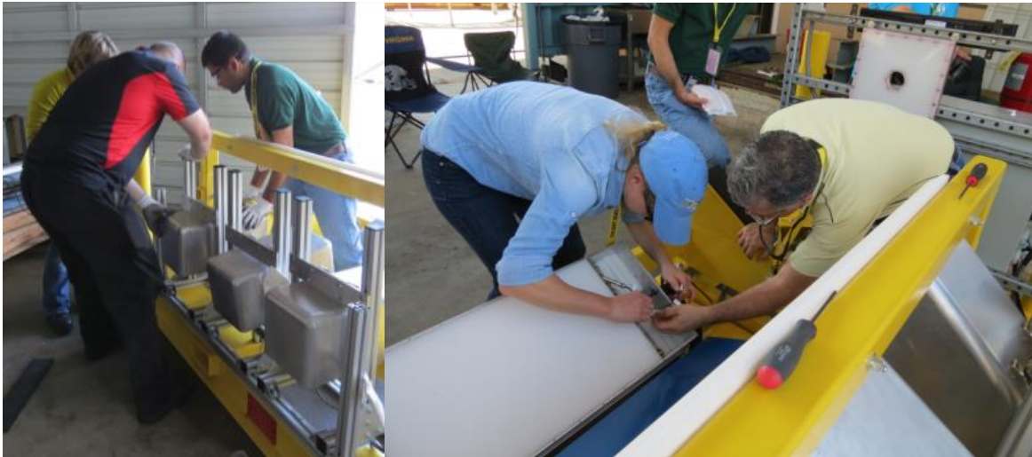
Figure 36. Installation of the HEVA (left) and PNEM (right) NDA modules on the platform.
