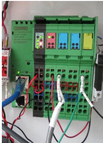
Figure 21. Phoenix Contact remote input output module with extra analog output terminal block.
