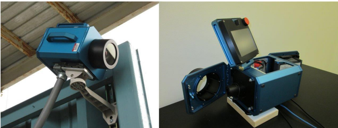
Figure 25. Deployment location for the area surveillance camera (left) and NGSS (DCM-C5) camera shown with front back and top panels open (right).
