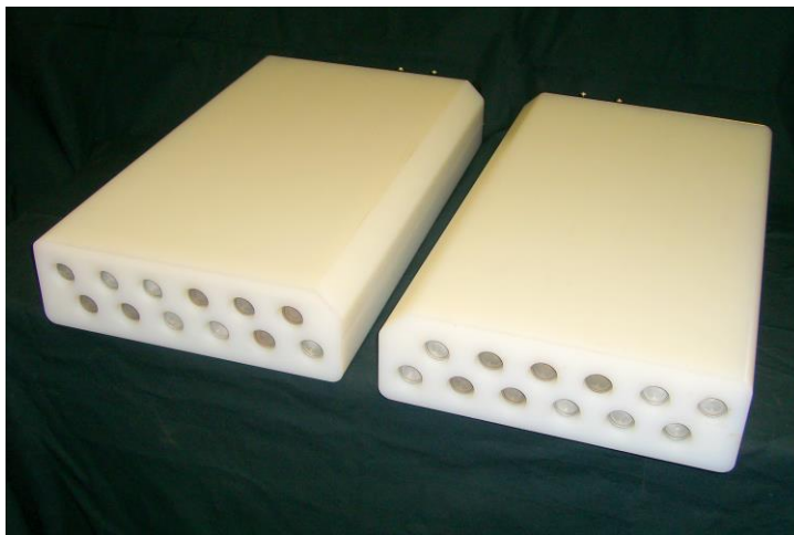
Figure 17. Photograph of the PNEM detector pods, each containing 12 10-atm ^3\text{He} tubes and weighing 17.6 kg.
