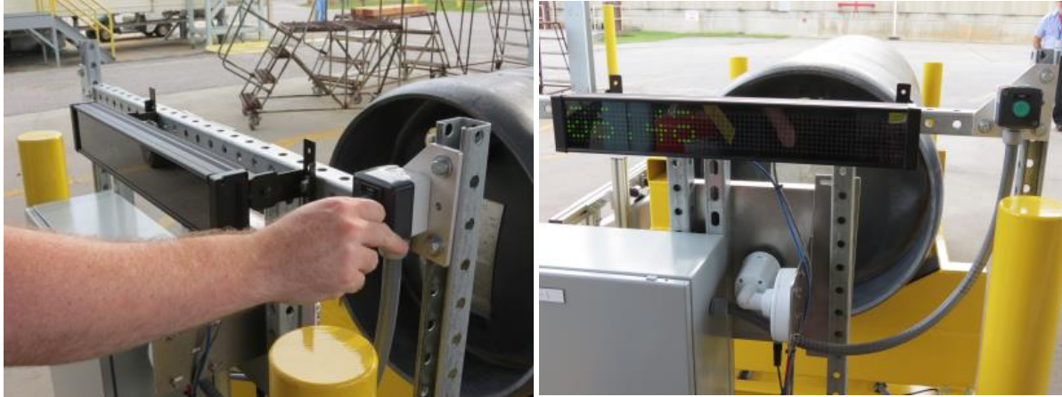
Figure 40. Initiate cylinder assay using the green START button on the UCVS assay platform. The remaining assay time is displayed on the digital display.
