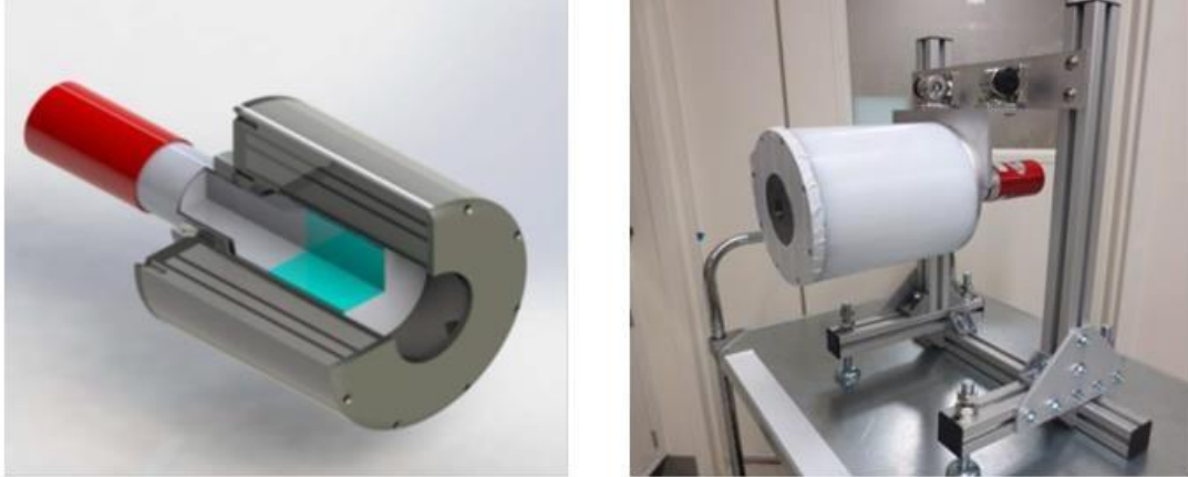
Figure 9. Left: Cross-sectional rendering of the HEVA detector-collimator assembly. The Osprey digital tube base is depicted in red on the left, the NaI(Tl) crystal is the light blue object. Surrounding the crystal are layers of lead, polyethylene, and steel to manage the total count rate and enhance neutron-to-gamma conversion. Right: Photograph of the mechanical support for a HEVA module that allows flexibility in terms of orientation angle relative to the cylinder face.
