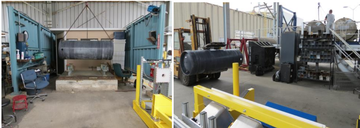
Figure 41. Left: Once the remaining assay time has expired, remove the cylinder from the UCVS assay platform and transfer it to the accountability scale using the overhead crane. Right: Remove the cylinder from the accountability scale using the fork truck before placing the next cylinder on the UCVS assay platform. Removal of the cylinder from the scale before, rather than during, the next UCVS occupancy prevents radiation background variation.
