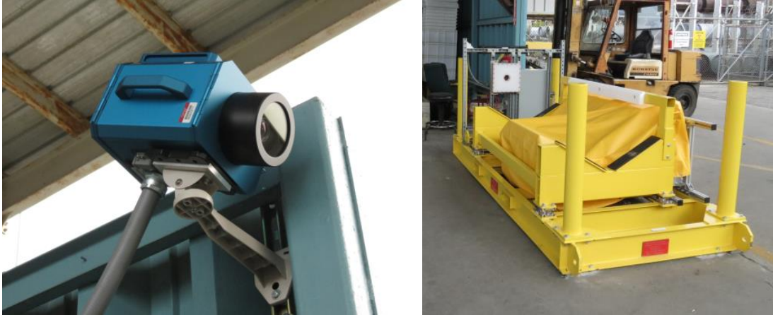
Figure 38. Area surveillance camera mounted on the curtain wall (left); environmental cover intended for placement on UCVS after each measurement sequence is completed (right).
