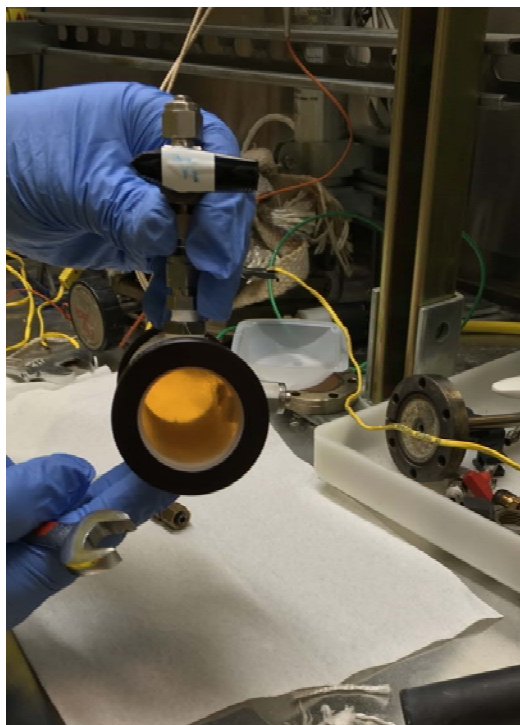
Figure 5. Photograph of Gas Sample Cell, Showing Visual Evidence of Presence of NO x Gases (orange color)
