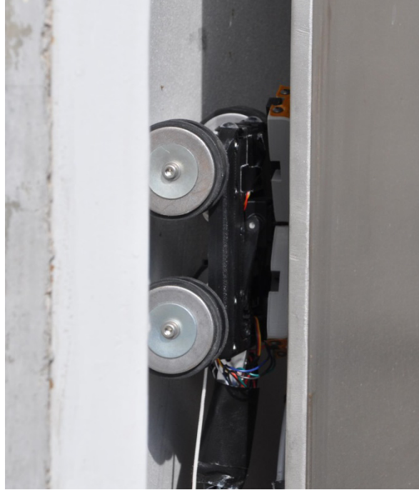
Figure 2.81. Photograph of a Robotic Delivery System Located Between the Stainless Steel Canister and Overpack of a Cut-Away Dry Storage Cask System at the Palo Verde Energy Education Center – Buckeye, Arizona (EPRI 2016). Reprinted with permission of the Electric Power Research Institute.
