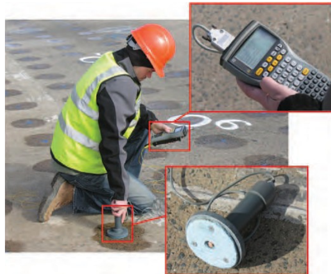
Figure 2.29. LPR Testing Conducted in the Field (TRB 2013, pp. 22-24)
