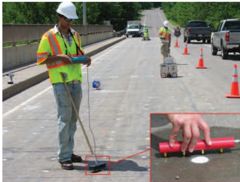
Figure 2.31. Photograph of Application of the Four-Probe (Wenner probe) Method in the Field (TRB 2013, pp. 24-25)
