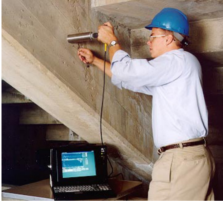
Figure 2.4. Photograph Depicting the Implementation of Commercial Impact-Echo Testing Equipment (With permission of Impact-Echo Instruments, LLC a )
