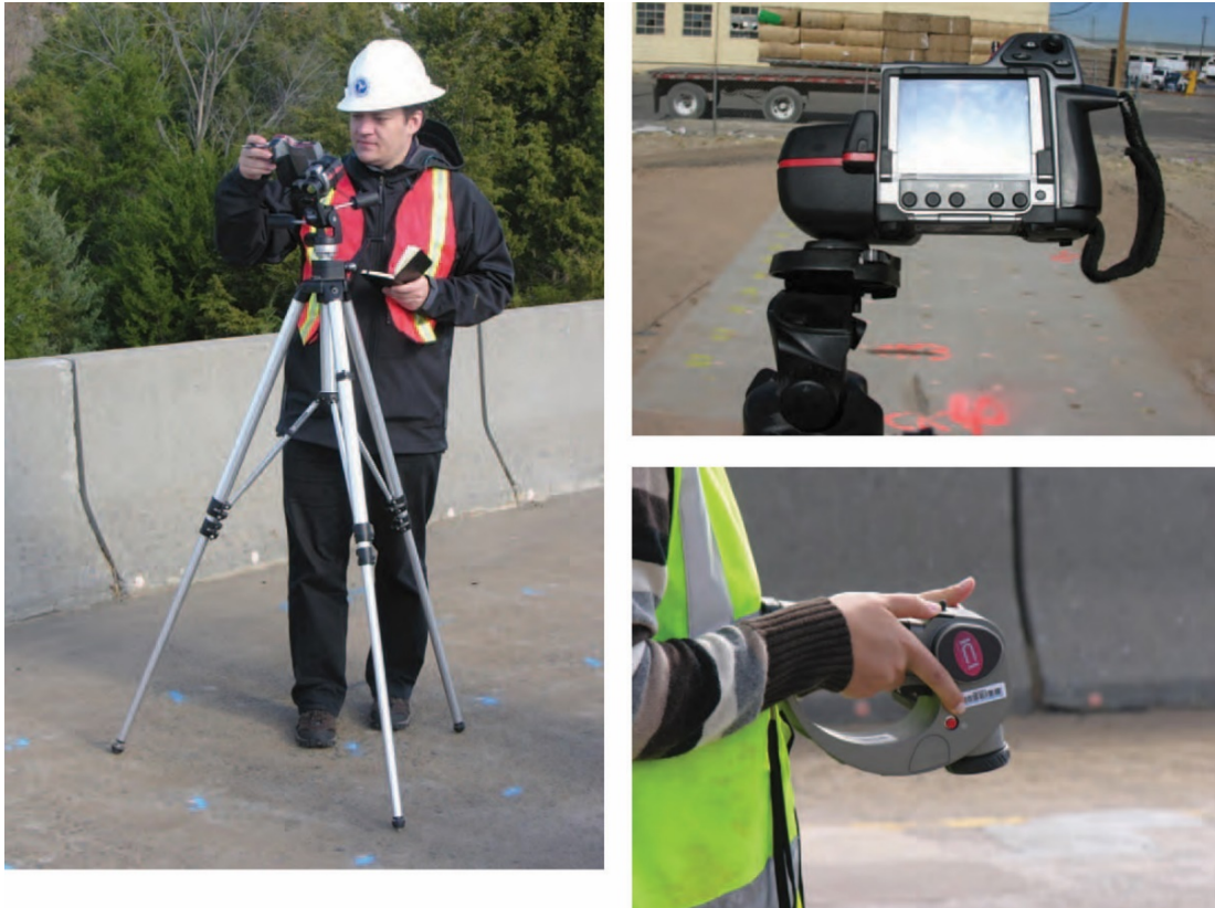
Figure 2.16. Depiction of IRT Testing on a Bridge Deck (TRB 2013, pp. 25-27)
