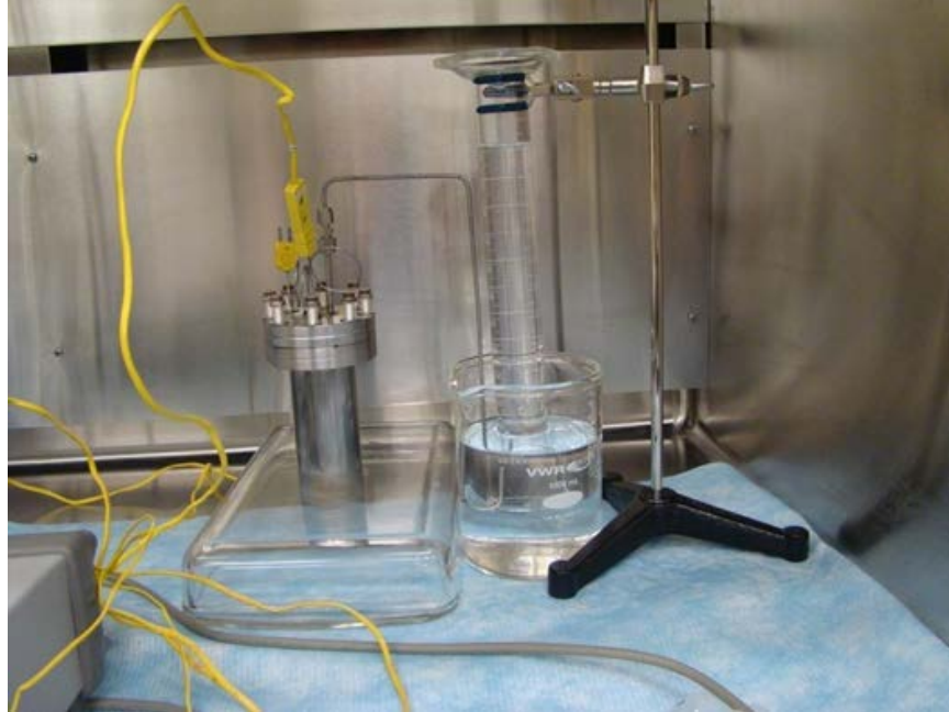
Figure 6.13. Stainless Steel Vessel Used for Simulant Temperature Testing
