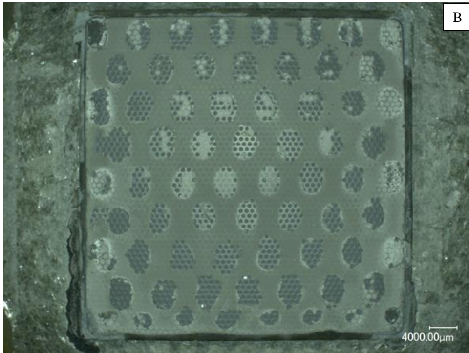
Figure 10. Post-test analysis of cell #140 with surface-blasted (grit #40), spinel-coated AISI441 interconnect after long-term test at 800°C: (A) anode side of the interconnect, and (B) anode side of cell. Both sides showed typical gray color of reduced Ni without any discoloration, consistent with hermetic sealing, as indicated from lack of cross-bubbling at room temperature.
