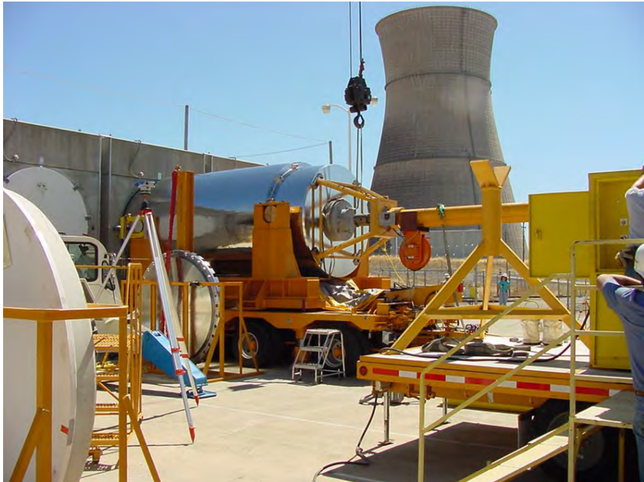
Figure 2-83. MP187 Transportation Cask and Hydraulic Ram Being Used to Load a Canister into a Horizontal Storage Module at Rancho Seco
