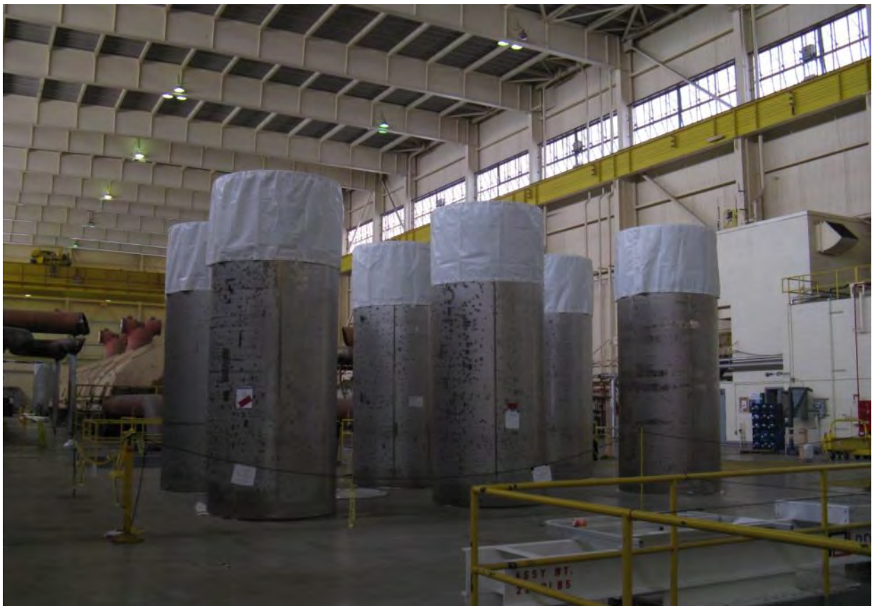
Figure 2-135. Used Nuclear Fuel Transportable Storage Canisters Staged at Zion (2013)
