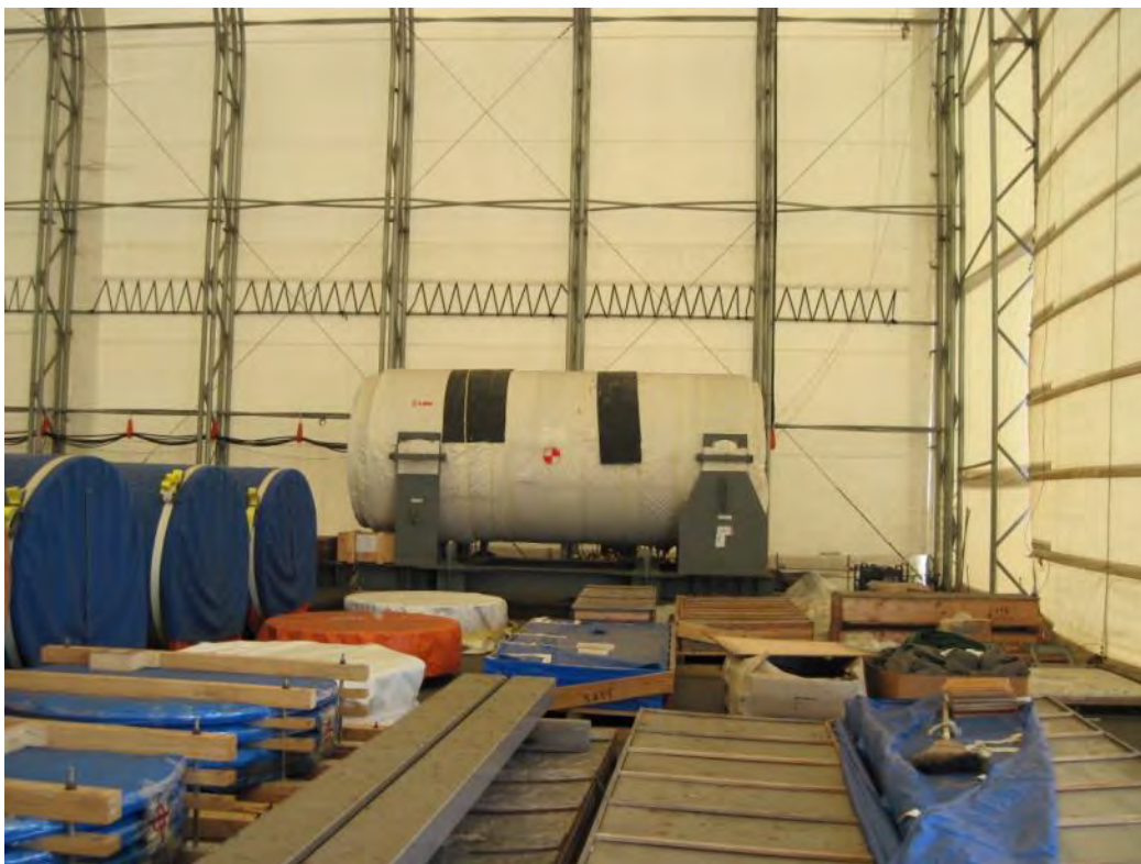
Figure 2-258. Transfer Cask for 32PTH2 Canisters (2015)
