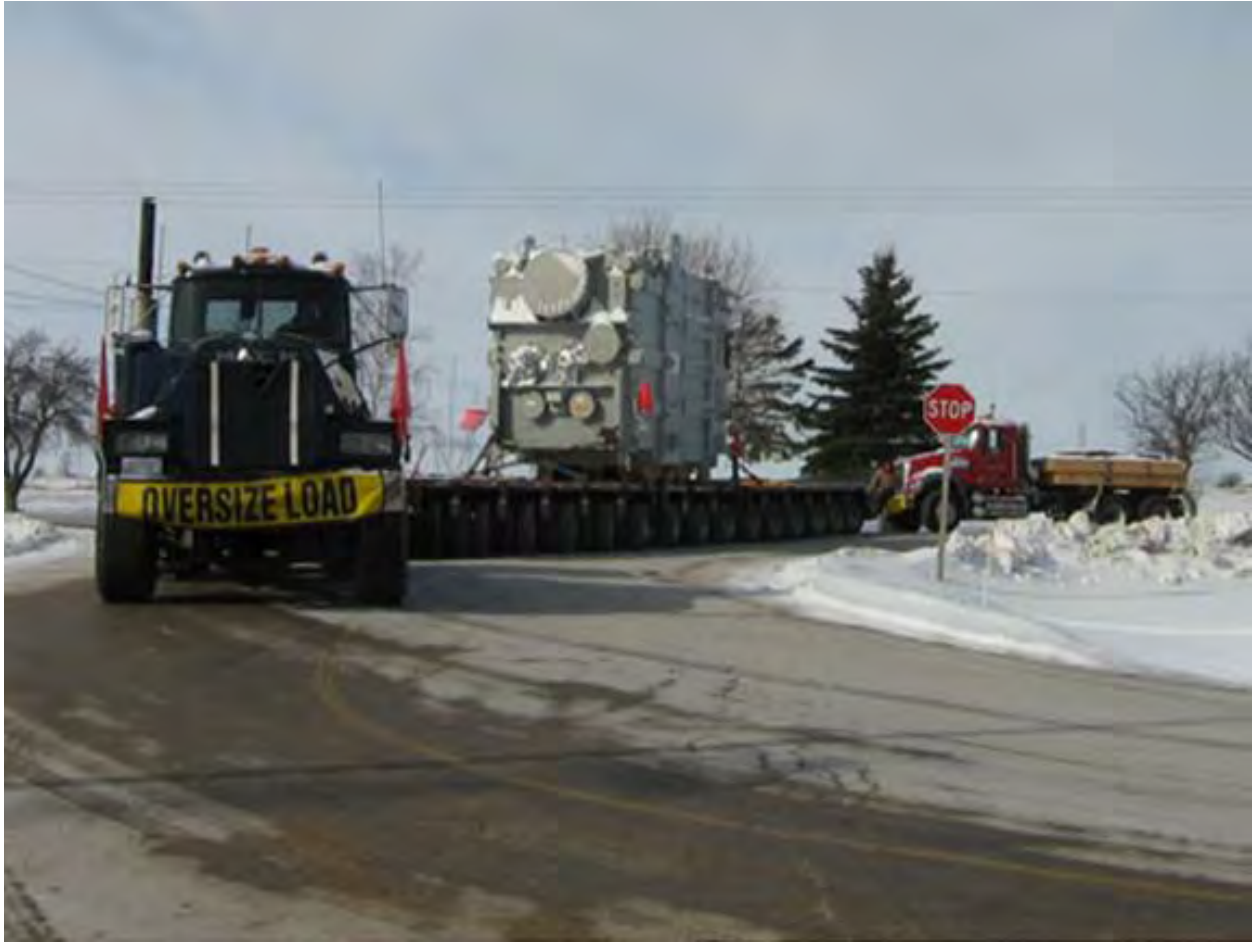
Figure 2-207. Transformer on 15-axle Goldhofer Trailer (2008)
