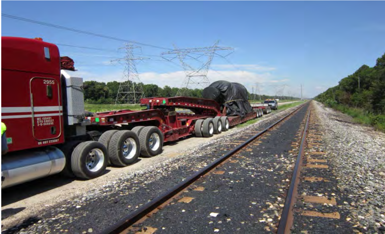
Figure 2-191. High Pressure Turbine Rotor Delivered to Crystal River Site by Heavy Haul Truck (2011)
