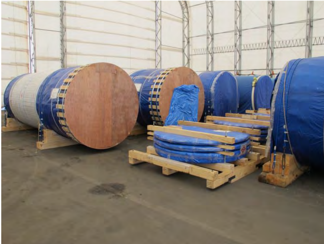
Figure 2-257. 32PTH2 Dry Storage Canisters (On Left) (2015)
