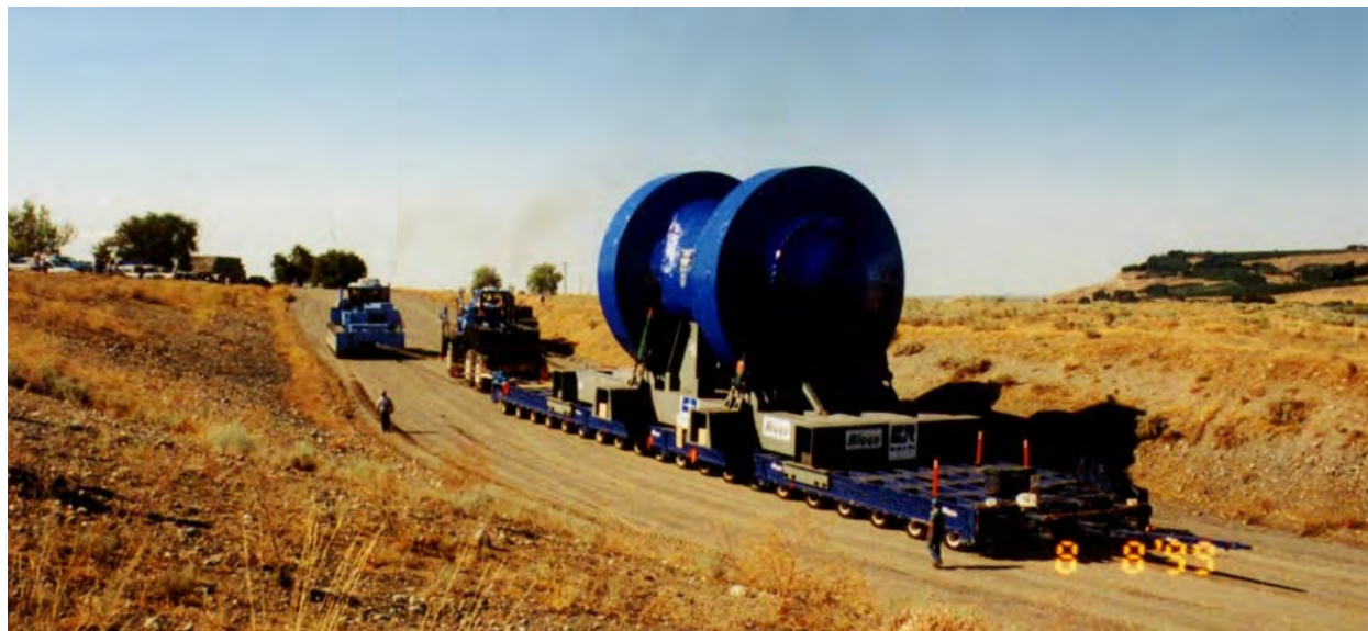
Figure 2-112. Trojan Reactor Pressure Vessel Being Transported by Heavy Haul Truck (1999)
