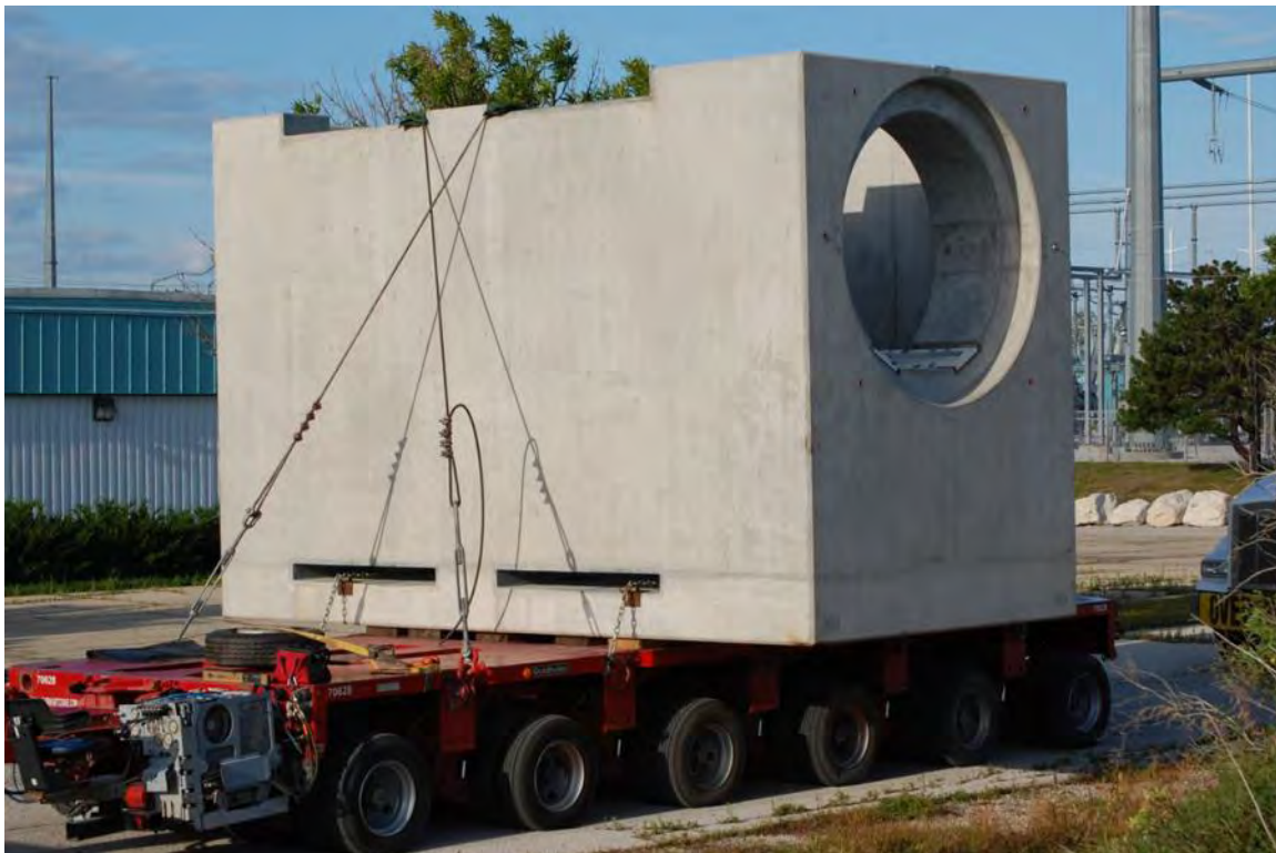
Figure 2-244. Horizontal Storage Module on 6-axle Goldhofer Trailer (2013)
