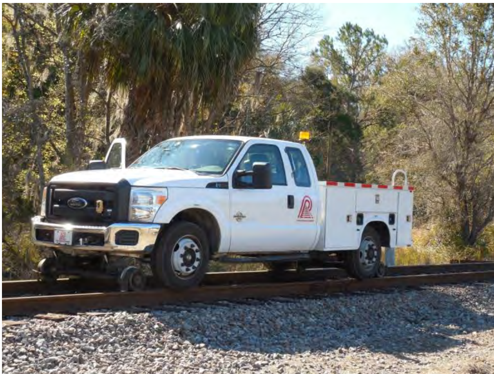
Figure 2-171. Hi-Rail Vehicle Used for Track Inspections (2015)
