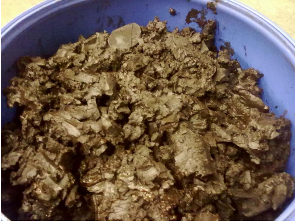
Figure 3.7. Iron-Rich Solids at Vendor After Concentration in Basket Centrifuge
