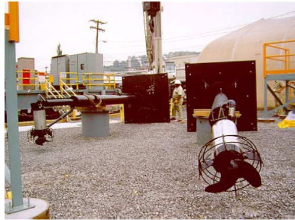
Figure 5.1 View of Russian pulsating mixer pump in tank TH-4 (left) and Flygt mixers on top of tank W-5 (right) before deployment
