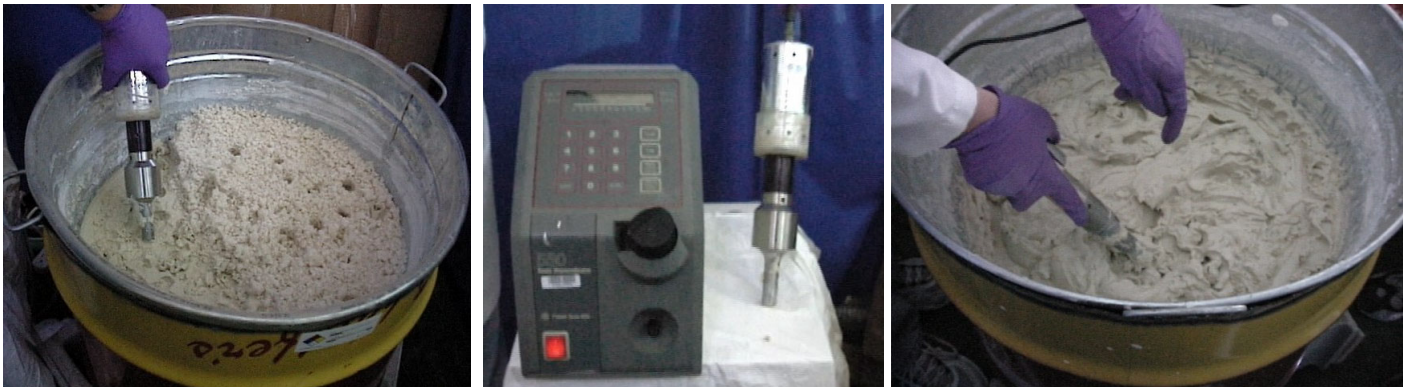
Figure 4.2 Sonicator system and dislodging of salt cake and sludge simulant
