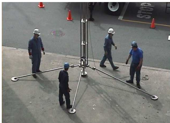
Figure 5.2 View of Pulse-Air mixer before deployment in tank W-9 and pulsed jet fluidic mixer at Bethel Valley Evaporator Service Tanks
