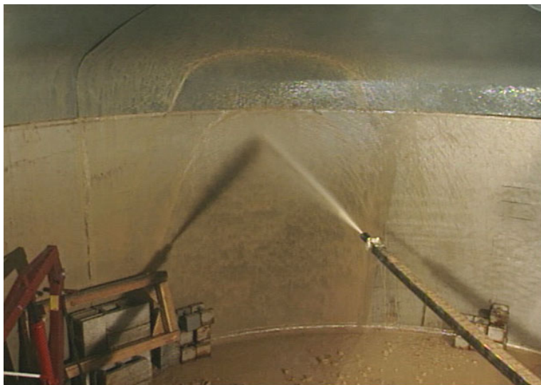
Figure 4.6 Testing of the borehole miner showing the focused movable nozzle and linked arm
