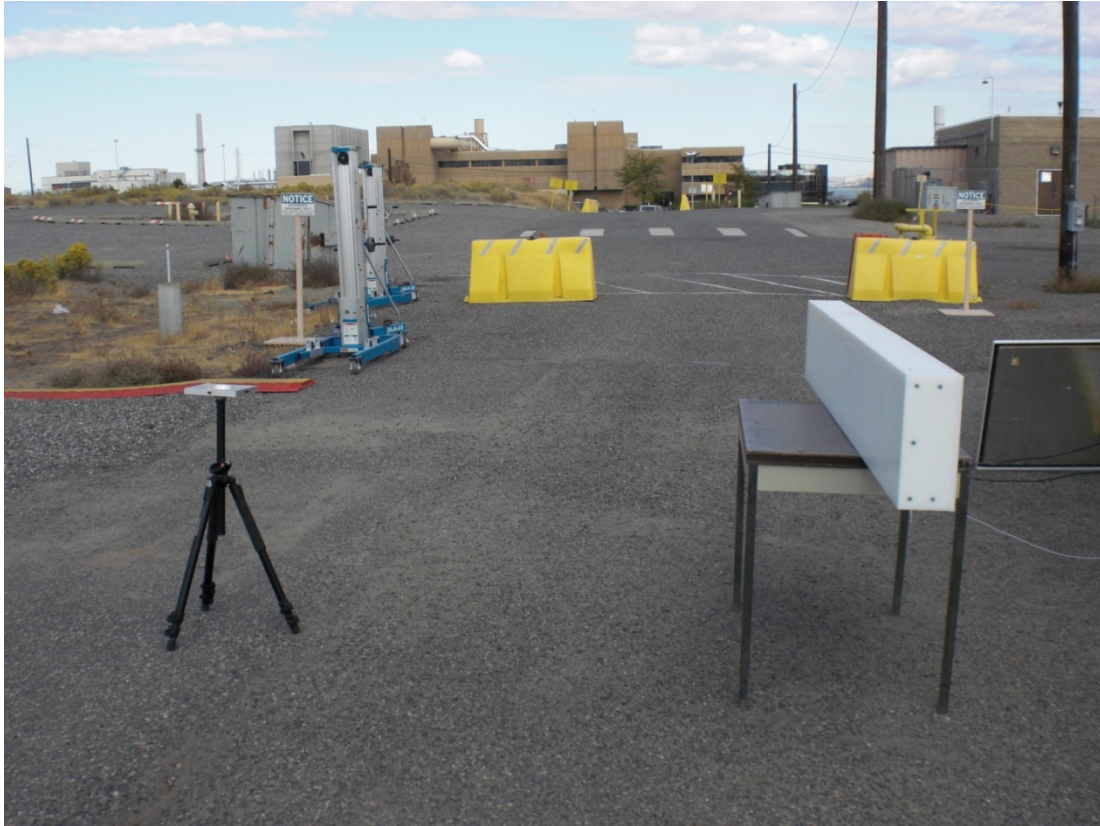
Figure 5.1: GE Reuter Stokes detector assembly positioned for static tests outside of the SAIC shroud.
