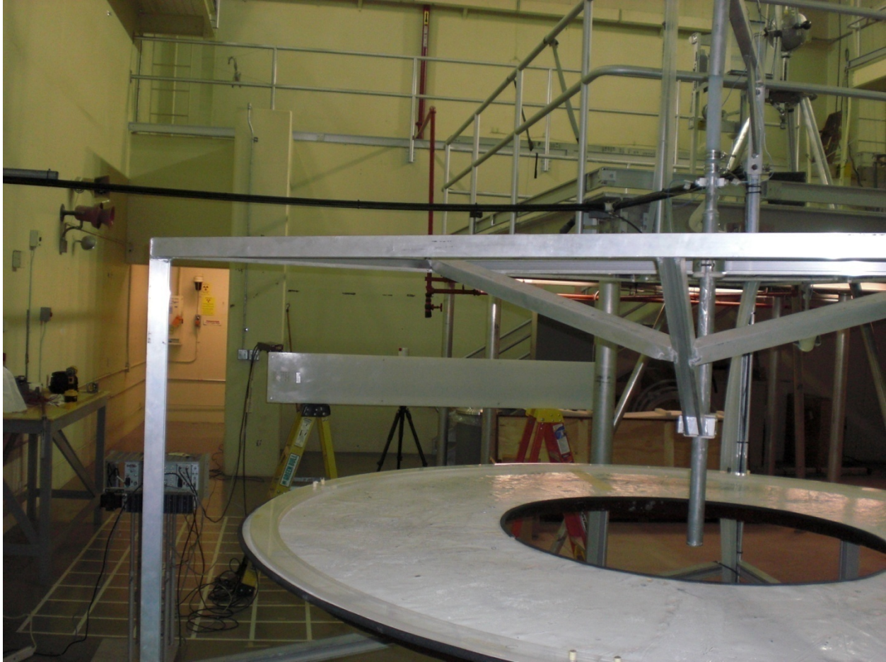
Figure 5.2: GE Reuter Stokes detector positioned for testing with the gamma ray and neutron sources.
