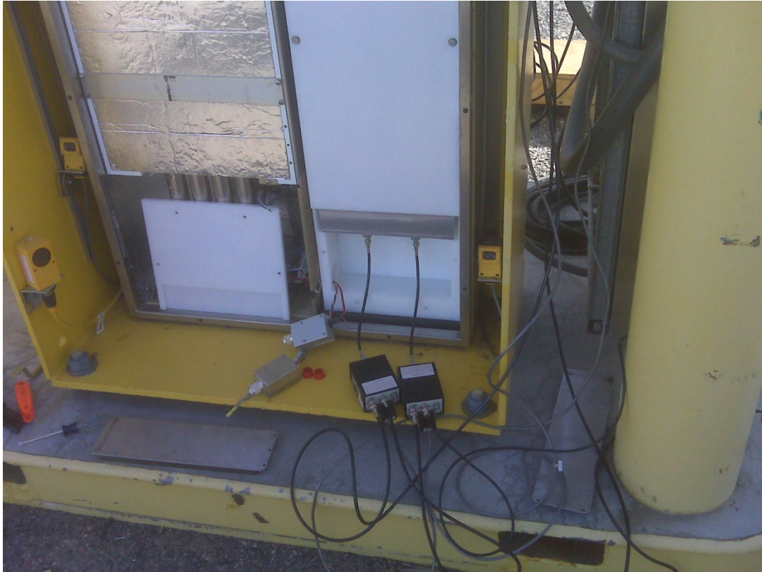
Figure 3.2: GE Reuter Stokes external detector electronics used in the testing.
