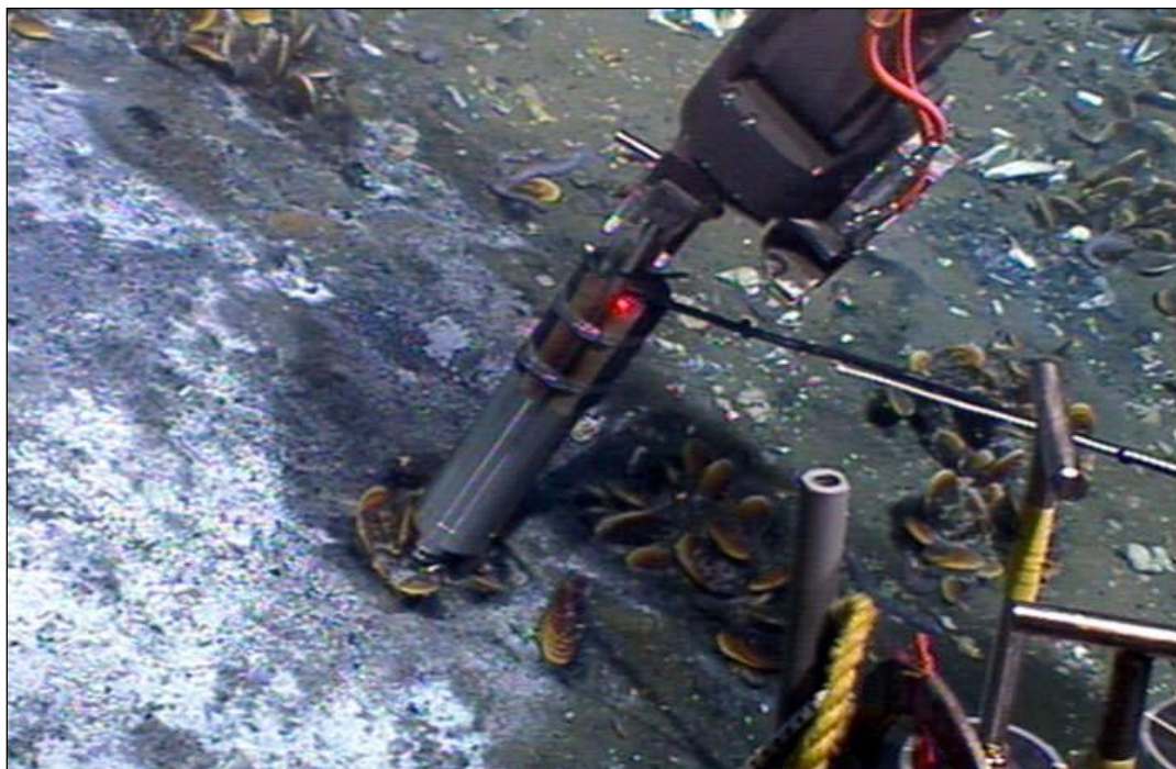
Figure 10-22. Testing CONTROS Methane Sensor near bacterial mat.
