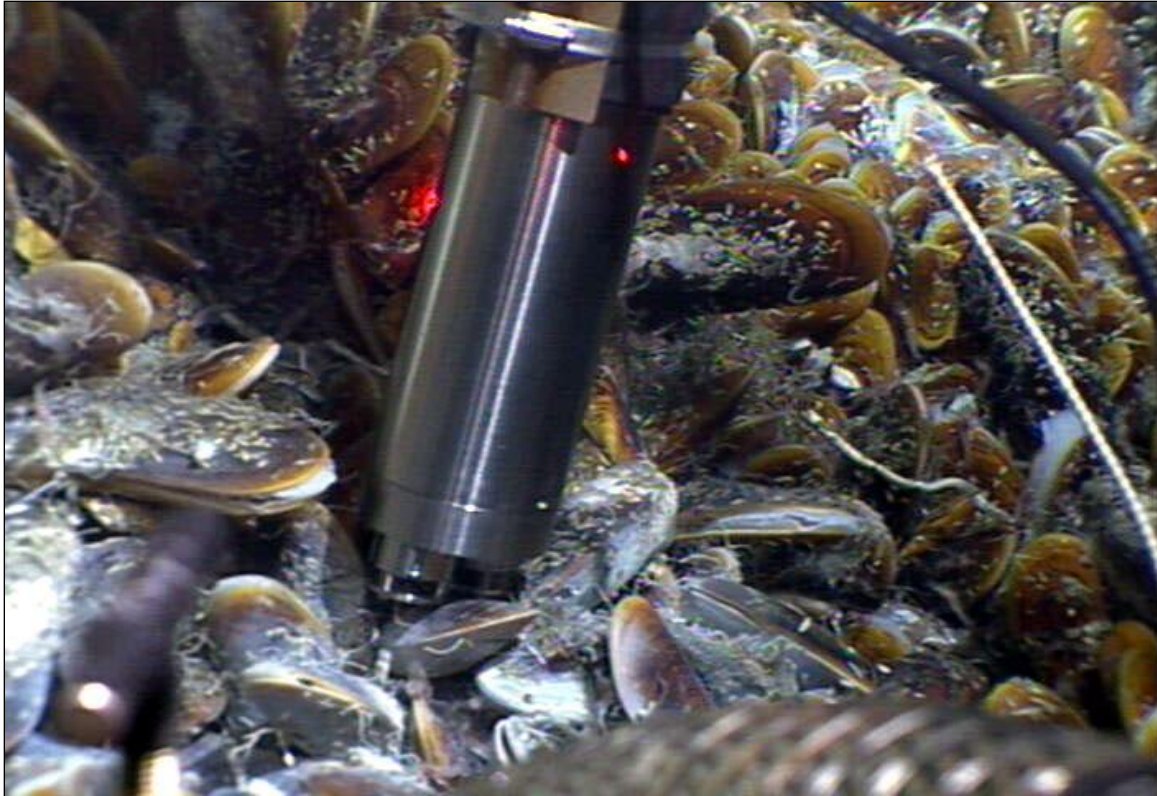
Figure 10-23. Methane Sensor deployed in mussel bed.
