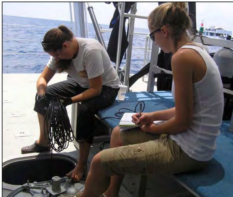
Figure 9.2.3. FGBNMS researchers conducting seawater temperature profiles using a YSI probe through the moon pool of the R/V Manta (NOAA/FGBNMS).
