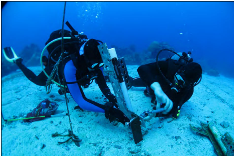
Figure 9.2.2. FGBNMS research divers mounting the Sea-Bird 37-SMP MicroCAT water quality instrument on a rack in the sand at the EFGB (NOAA/FGBNMS).
