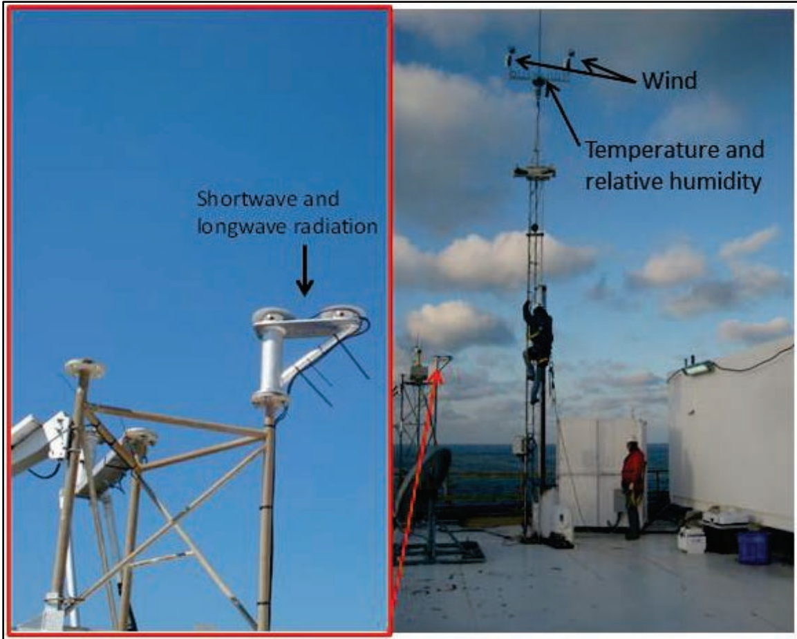
Figure 7. Shortwave and longwave radiation and surface meteorological tower on Chevron's ST-52B oil platform in the Gulf of Mexico.
