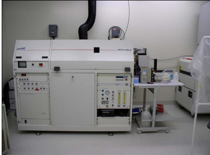
Figure 8. Fisons/VG PlasmaQuad® inductively coupled plasma-mass spectrometer used at the University of Hawaii at Manoa.
