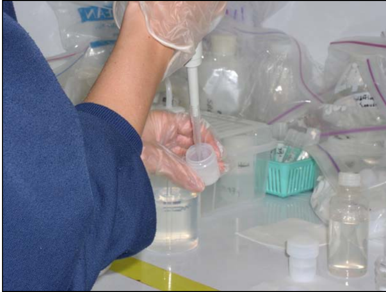
Figure 4. Addition of DI water to beakers and otoliths for rinsing off surface contaminants (Yvonne Perry—University of Hawaii at Manoa).
