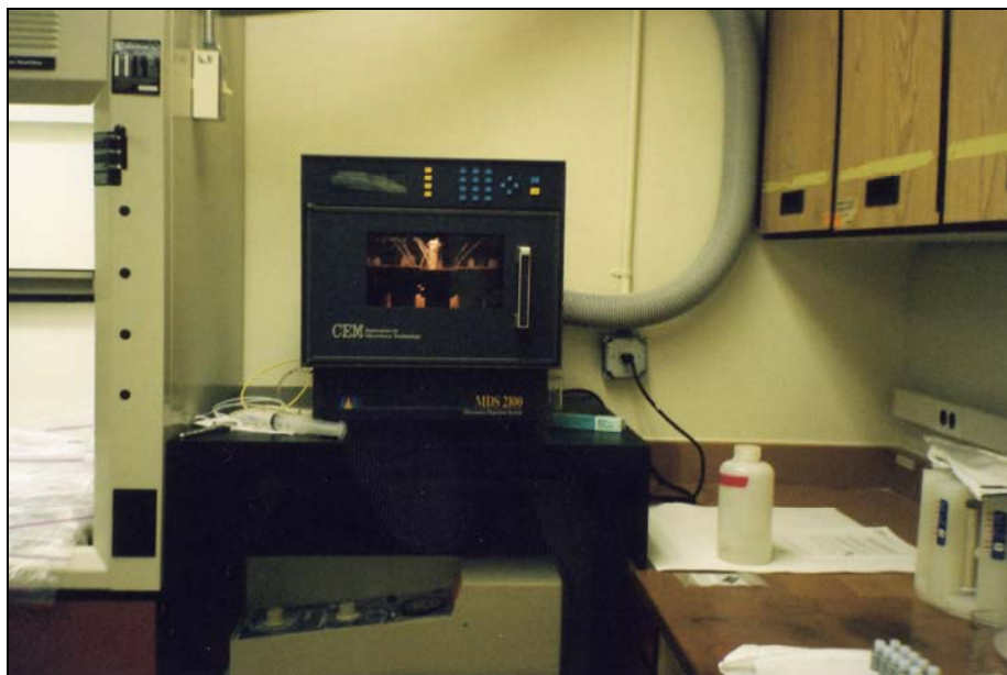
Figure 6. MDS 2100 Microwave Digestion System® used to dissolve otolith samples and blanks (University of Hawaii at Manoa).
