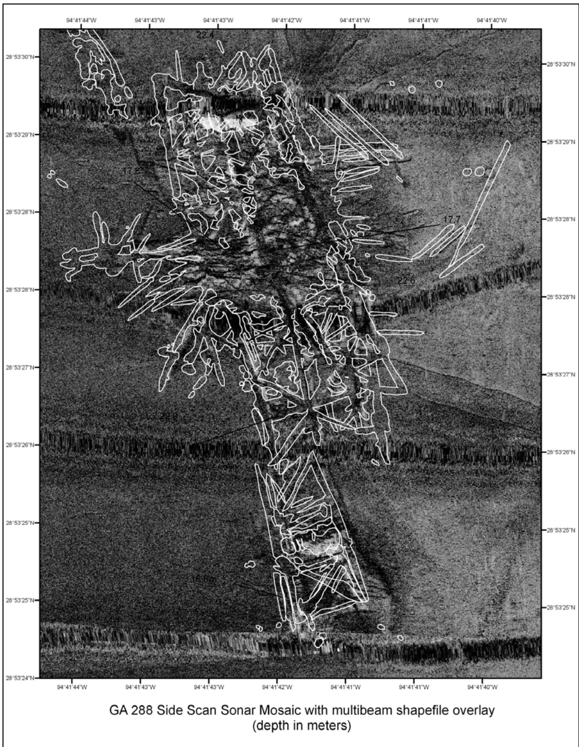
Figure A.13. GA-288 side-scan and MBES survey overlay; i.e., 2003 vs. 2005.
