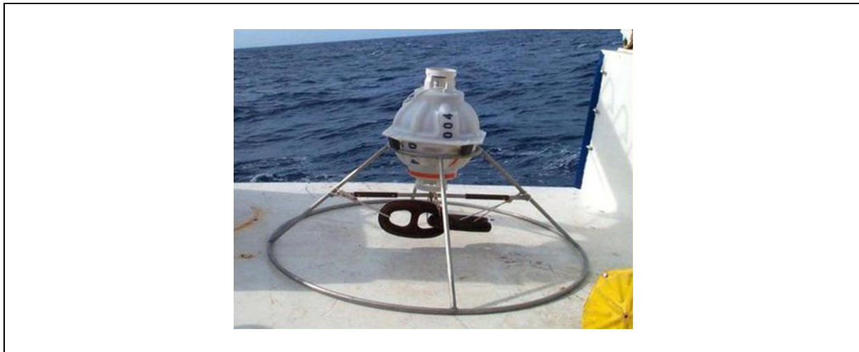
Figure 2I.15. The pressure-recording inverted echo sounder (PIES) is an ocean-bottom instrument housed in a single 17" glass sphere containing the controller/data logger, acoustic release, and relocation radio/strobe light. The PIES is released from the ocean bottom after it receives a coded acoustic command. The anchor stand is dropped; the PIES returns to the surface and emits an acoustic beacon—a relocation radio and a strobe flasher—for tracking.
