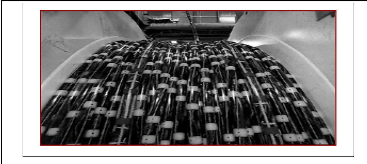
Figure 7. A streamer cable rolled up on a drum.
