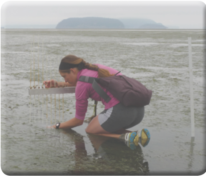
Figure 3.10 WWU graduate student and PBNERR research assistant Katrina Poppe taking measurements at a surface elevation table (SET) in Padilla Bay. Photo credit: Abe Lloyd.
