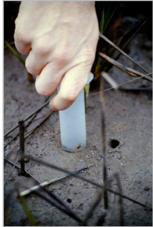
Benthic core sampling technique.
