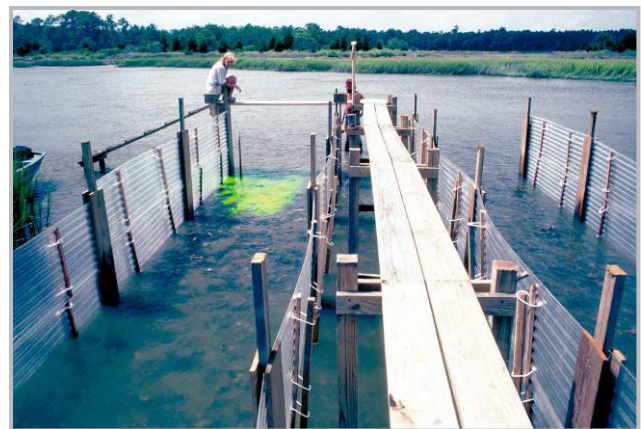
Flumes were used in Bly Creek to examine the transport of nutrients in the marsh.
