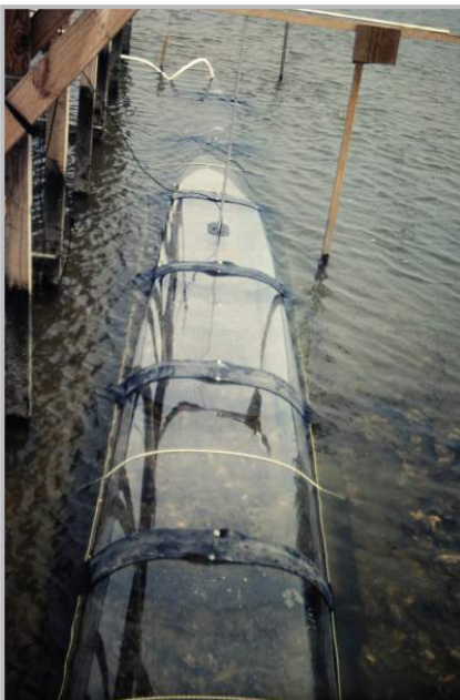
A 10 m long portable tunnel was used by Dame et al. to study nutrient flows over an oyster reef in Bly Creek.
