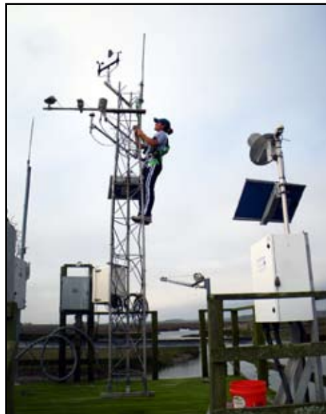
Meteorological conditions are measured every 5 seconds continuously throughout the year, producing averages for 15 minute, hourly, and daily data.
