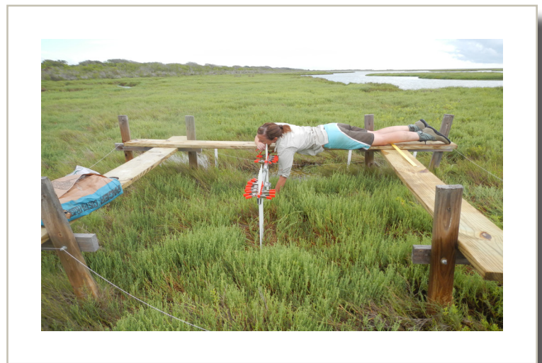
SETs are used to monitor changes in surface elevation at ANWR
