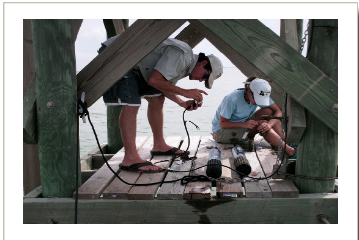
Research staff perform maintenance on water quality monitoring equipment at a SWMP station
