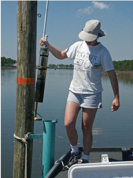
SWMP technician performing the monthly sonde rotation in Bayou Cumbest. Photo credit: Mark Woodrey.
