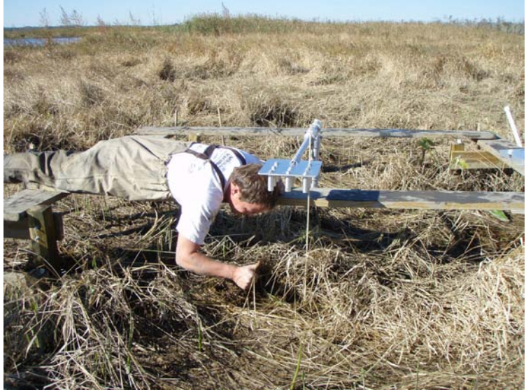
Figure 10.2. Deploying SET to measure sediment accretion on marsh surface. Photo credit: James Goins.
