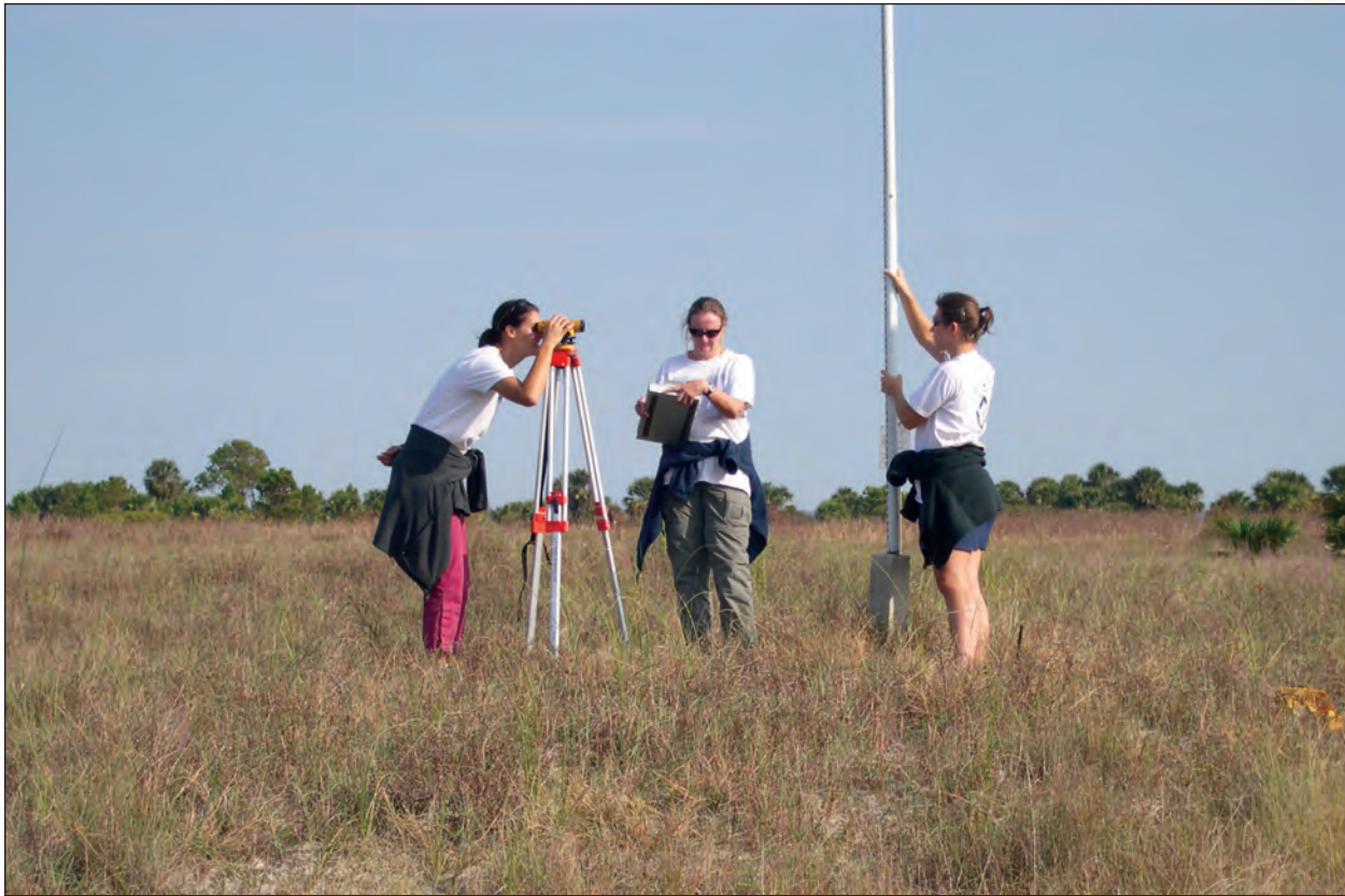
Reserve staff measuring dune elevation on Little St. George Island to calculate erosion and accretion rates.
