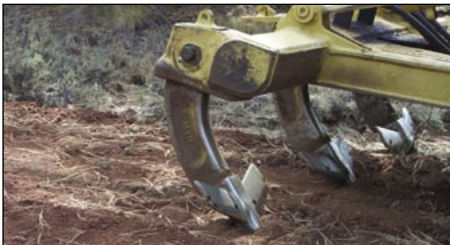
Figure 38—Larger equipment is used for deeper ripping to increase infiltration and break through water repellent soils.
