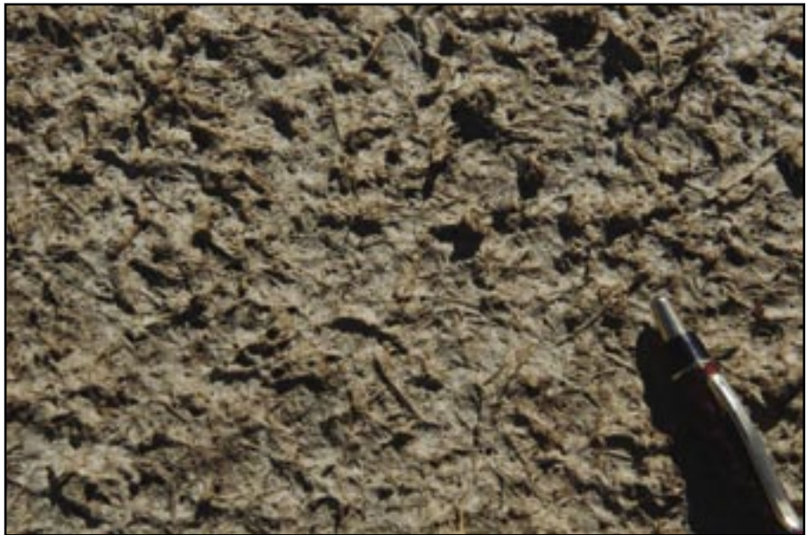
Figure 4—Hydromulch fibers form a smooth dense mat.
