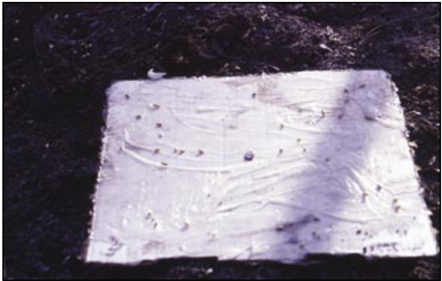
Figure 41—Validating the proper seeding rate with monitoring cards.
