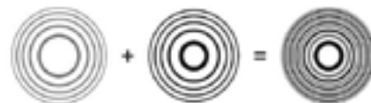
Schematic depiction of double-patterning process. (W. Chao et al., J. Vac. Sci. Technol. B 27 , 2606, 2009)
