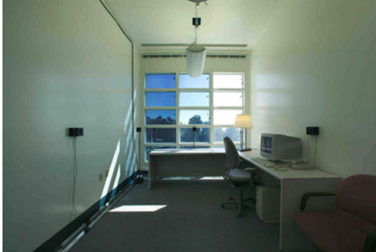
Figure 10-3 Switchable electrochromic windows provide variable solar, daylight, and glare control, shown at the LBNL Windows testbed facility. Source: http://lowenergyfacades.lbl.gov/technologies.html .
