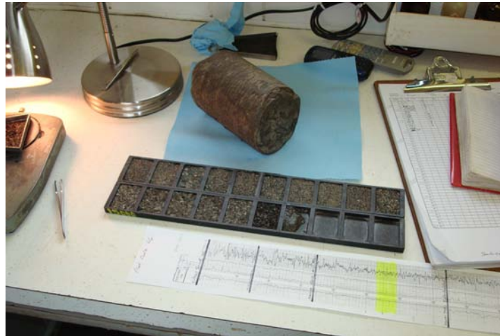
Figure 5-4 Drill cuttings and whole core collected for site characterization of geologic sequestration. Source: R. A. Esposito, Southern Company.
