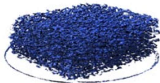
Figure 28 3-D Li distribution ( \text{Li}_2\text{O}_2 ) in coarser foam matrix, which can help to address interfacial transport and the Li transport in complex electrodes (degradation issues).
