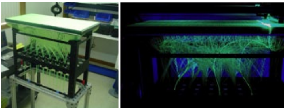
Figure 14 The WLS fiber detector, in daylight (left) and dark (right). The flat scintillator has an area of 77 × 38 cm 2 , and scintillation light is coupled by 308 and 152 fibers feeding 25 and 7 photomultipliers, respectively, for the X and Y axes.
