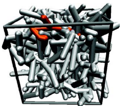
Figure 30. Snapshot from a coarse-grained simulation of an entangled DNA polymer system featuring flexible polymers in a computer-generated periodic box. The “test” molecule (orange) is undergoing close frictional interactions (entanglements) with the shaded molecules; thus the test chain is undergoing reptation or snake-like motion. The lighter chains are free of the test chain. Source: A. Dambal, A. Kushwaha, and E. S. G. Shaqfeh, “Slip-link simulations of entangled, finitely extensible, wormlike chains in shear flow,” Macromolecules 42 (18), 7168 (2009).
