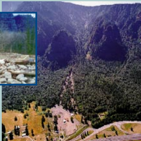
This debris flow occurred in the Columbia River gorge near the town of Dodson, Oregon, during a rainfall and snowmelt event in February 1996 (Photo Inset: S. Cannon, USGS). The combination of rainfall and snowmelt resulted in severe flooding and landsliding throughout the Pacific Northwest. The debris flow shown here was deposited in a number of separate events over a period of 2 days. The flows originated high on the palisade and traveled through the steep canyon. The occupants of the house escaped with their lives when they heard a loud rumbling and crashing of trees and saw the approaching material through their kitchen window. Boulders, mud, and debris from these and several nearby debris flows were deposited across the east-bound lanes of Interstate Highway 84, and blocked the highway for 5 days (Aerial Photo: D. Wieprecht, USGS).
