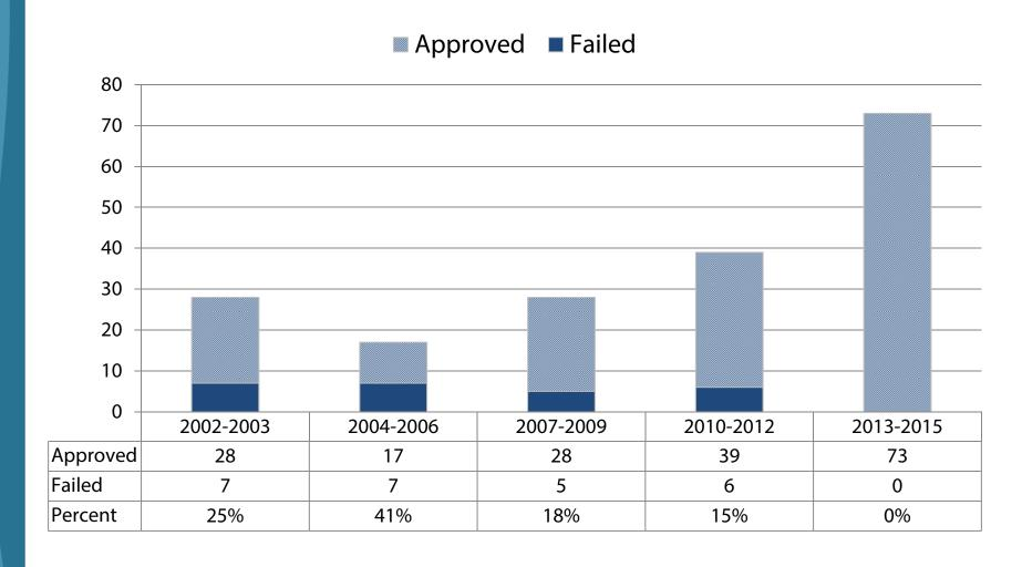
Total of 25 Known Failures of Approved MPFM/WGMs Several MPFM/WGMs (topside and subsea) from 2003 still in service
