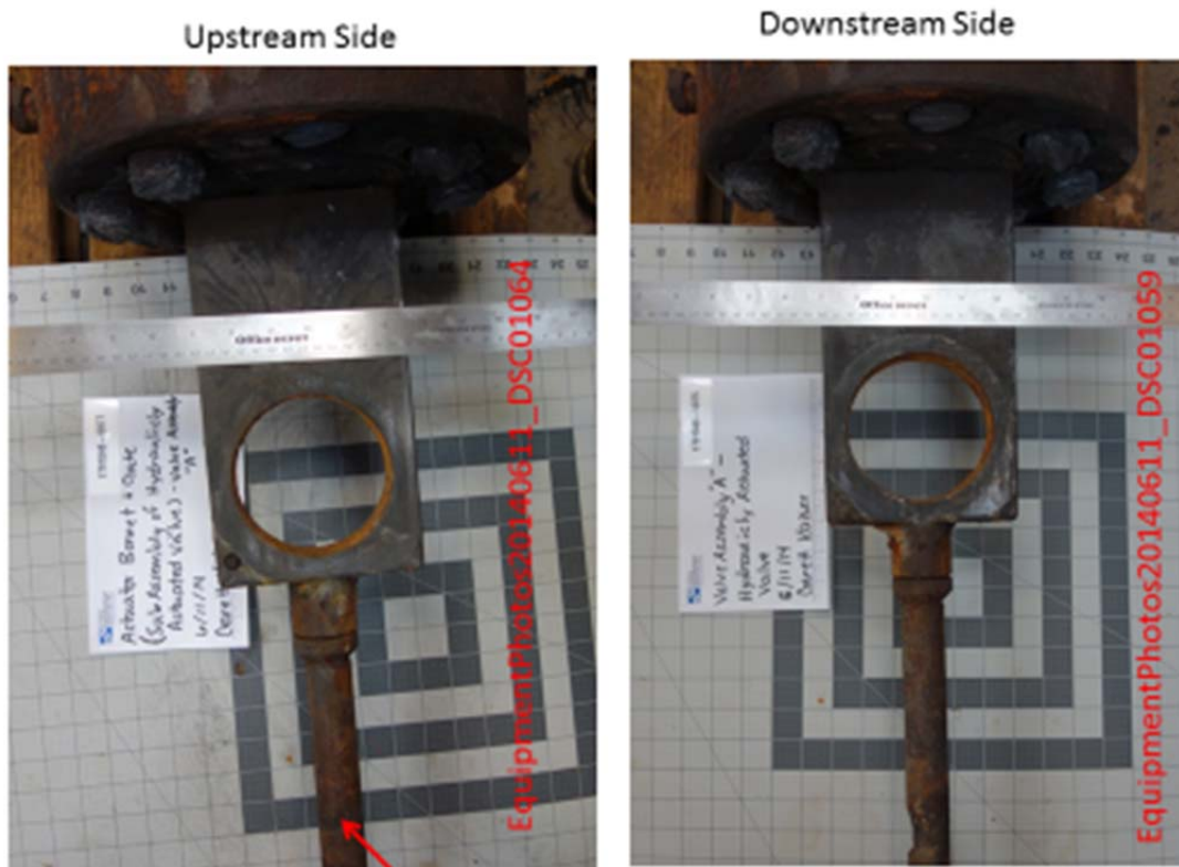
Figure 6.9 – Upstream and down-stream side of HCR valve gate as it was being removed
