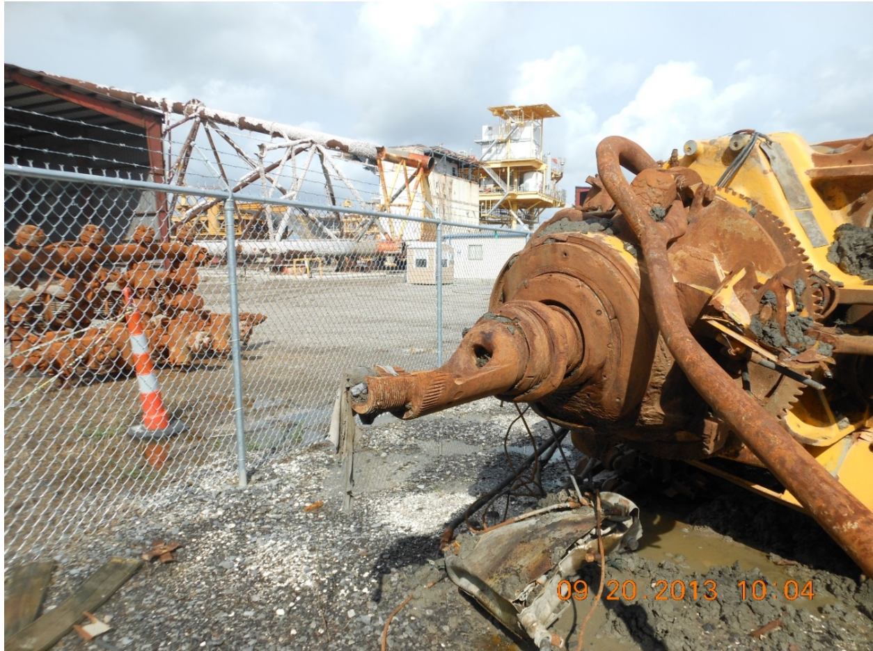
Figure 7.5 – Photograph of Bottom portion of Top Drive as recovered from Seafloor
