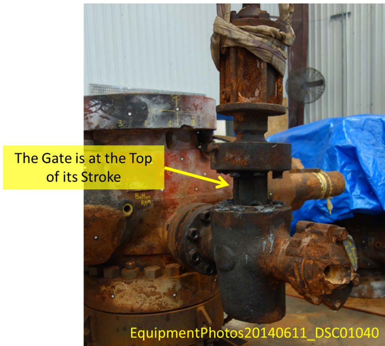
Figure 6.8 – HCR valve being disassembled at Stress Engineering
