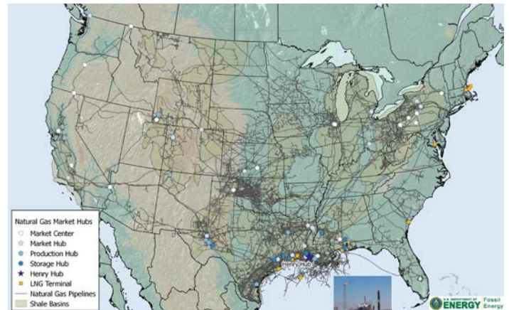
Figure 1. U.S. natural gas pipelines.
