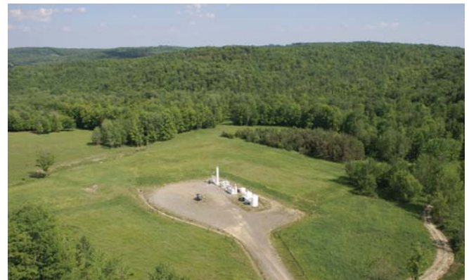
Figure 1. Shale gas well in the Appalachian Basin shows a well pad sited on a slope with an access road. The well pad siting and access road are examples of surface impacts that must be addressed.
