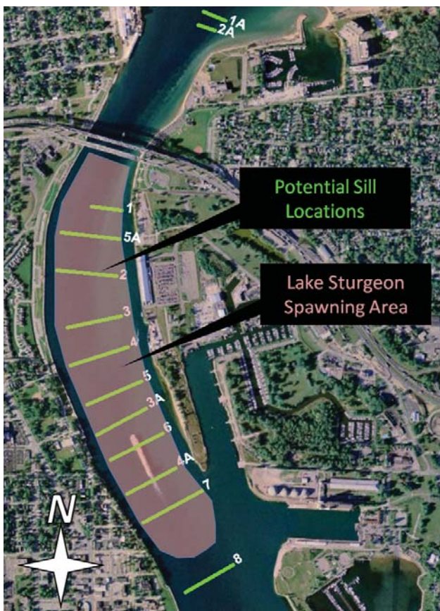
Figure 7-13 Overlapping Zone of Potential Sill Locations and Lake Sturgeon Spawning Habitat in the Upper St. Clair River
