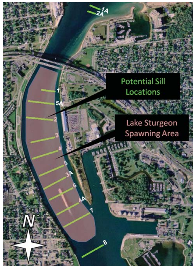
Figure 11-6 Overlapping Zone of Potential Sill Locations and Lake Sturgeon Spawning Habitat in the Upper St. Clair River
