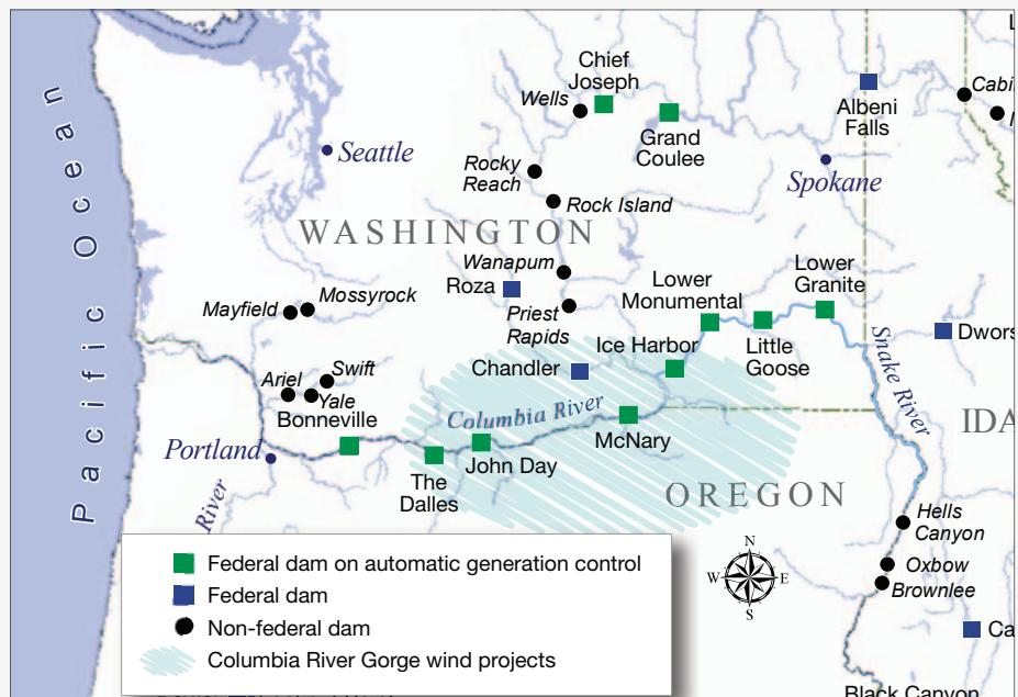
*Automatic Generation Control allows federal hydro operators to use the lower Snake River dams to meet loads minute-to-minute while using the Columbia River dams to support wind power. There are 31 federal dams in the Columbia Basin; the 10 largest have AGC capability.*
