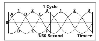
The three phases give each AC cycle three positive peaks and three negative valleys. To convert this power to DC, at each peak, one mercury arc valve or half of a thyristor valve picks off the positive pulses.
