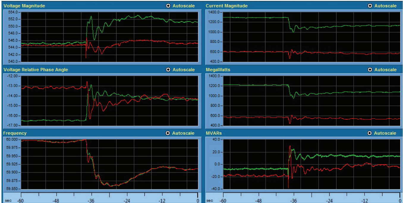
PMUs measure voltage, current and frequency in real time using time-synchronized GPS. This synchrophasor data stream shows what BPA operators saw when a power plant tripped and triggered a disruption across BPA's power system.
