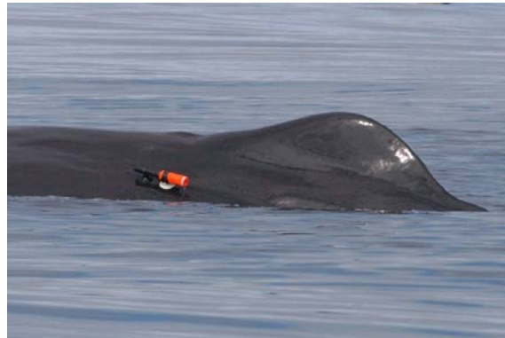
Figure 2. Bioacoustic tag attached to a sperm whale in the Eastern Gulf of Alaska
