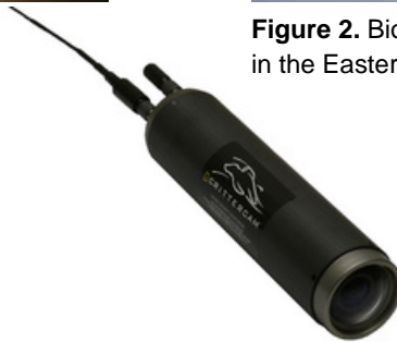
Figure 4. Crittercam Generation 5.7, bioacoustic and video camera suction cup tag.
