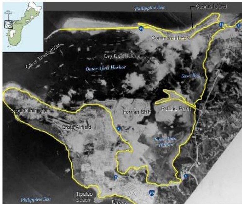
Figure 18. Apra Harbor July 1945. The yellow line indicates the approximate shoreline prior to the dredging and fill projects of the 1940s.
