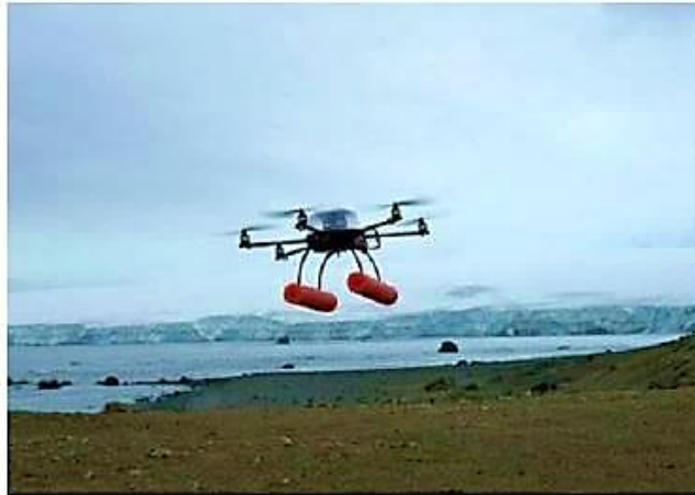
Figure 4: One type of unmanned aerial system that has been used in the field by NOAA/NMFS personnel for marine mammal research: the APH-22 Hexa-copter.
