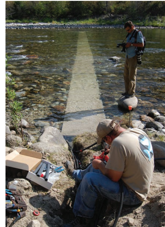
A technician wires a PIT tag antenna stretching across the remote South Fork of the Salmon River in Idaho to a telemetry station that can beam data to scientists. The antenna is among the largest of its kind.
