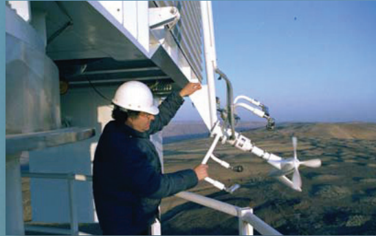
A project engineer inspects anemometers and other sensitive instruments that feed data to computers controlling operation of a MOD-2 unit. (NASA)
