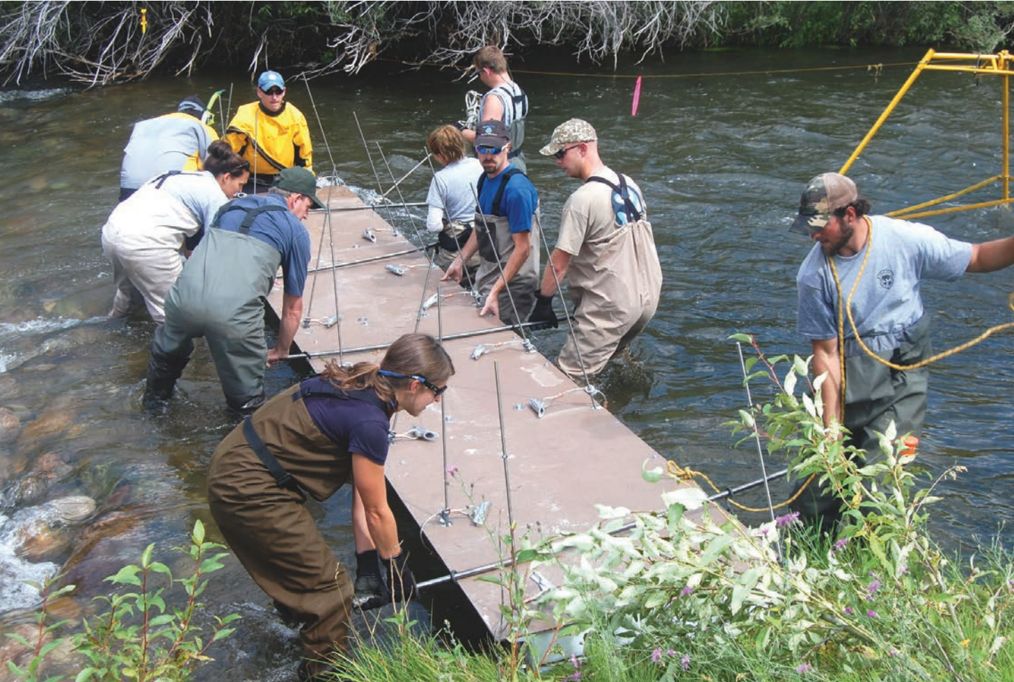
A team, including one person with a snorkel and dry suit, anchors a PIT tag antenna on the bottom of Idaho's Lemhi River in 1989.
