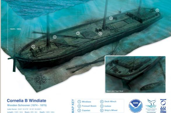
Wooden Schooner (1874 - 1875) Lake Huron (N45\* 00.976' W 83\* 09.899\*) Length: 138ft / 42m Beam: 26ft / 8m Depth: 190ft / 58m
