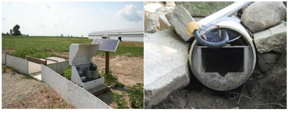
Figure 1: Edge-of-field surface runoff site with a 2.5 foot H-flume
