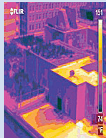
Figure: This infrared image, with a temperature scale on the right, reveals that “green” roofs are cooler (darker in color) than the surrounding conventional roofs. Image courtesy of Chicago Police Department and the Cook County Sheriff’s Department.
