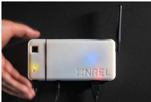
IPOS detectors combine smartphone technology and open-source recognition software to detect movement in a room with an accuracy of more than 90 percent. (Photo by Dennis Schroeder, NREL)
