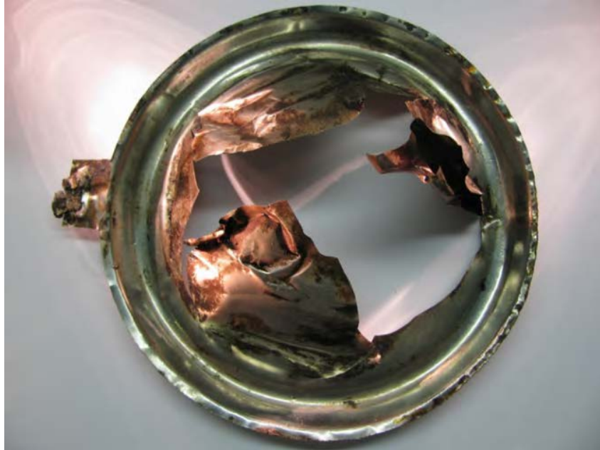
Fig. 6 – Rupture Disc (PSE) Recovered from Houchin Surge Tank One (BSEE Photo)
