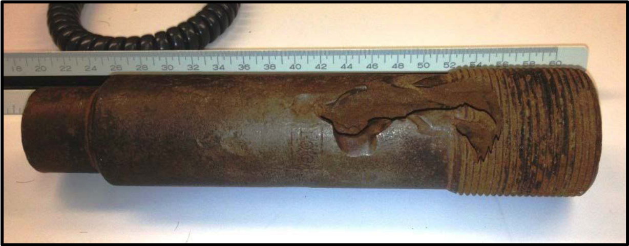
Figure 45: Choke body eroded from high delta P and micro-fines (2)
