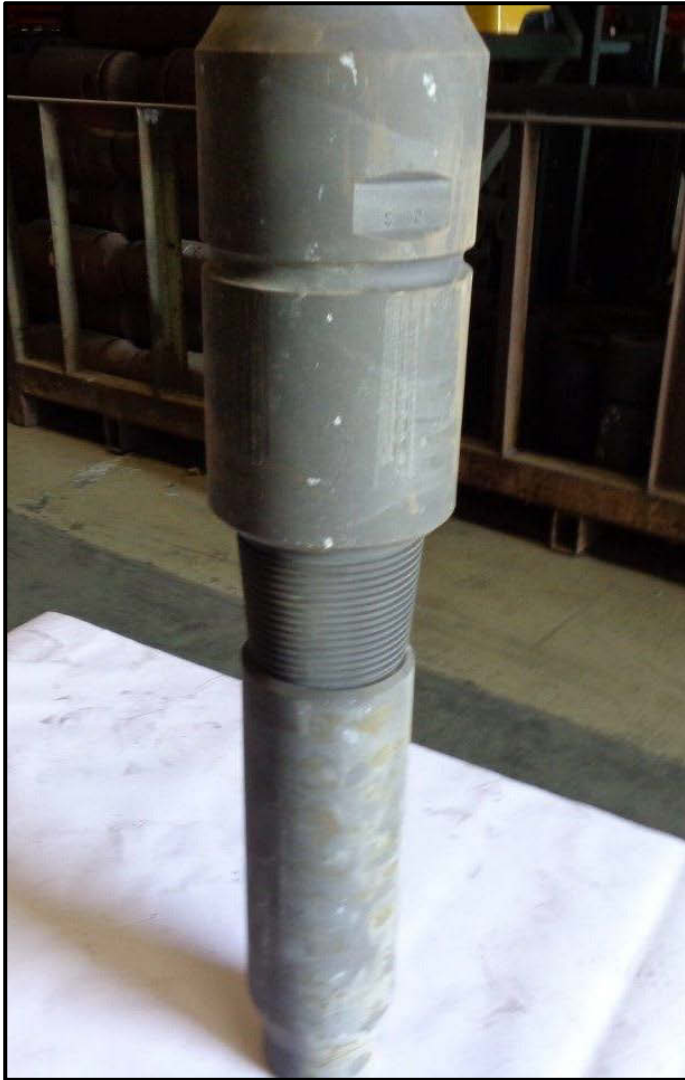
Figure 22: Top drive 5-in pin above 3 ½-in box
