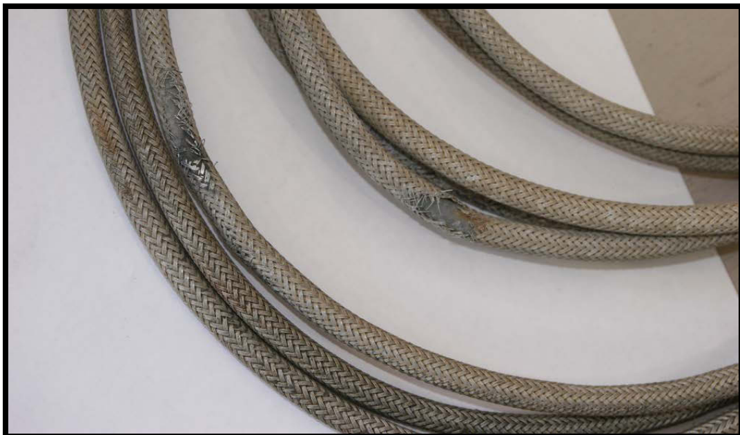
Figure 22: Armor Condition of Extension Cord
