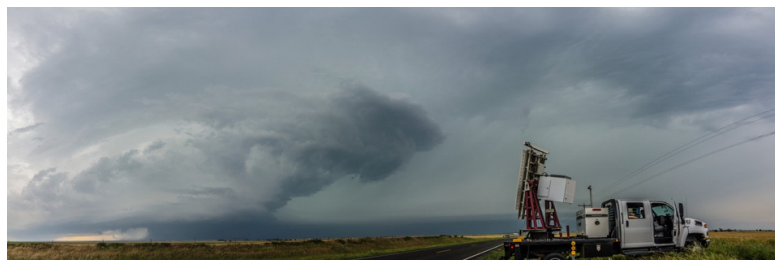
A Plains Elevated Convection at Night (PECAN) mobile observing station. The PECAN campaign focused on characterizing conditions that lead to nighttime storm formulation over the Great Plains, in order to improve the ability of climate models to make long-term projections about precipitation and hydrology. (Source: James Kurdzo).
